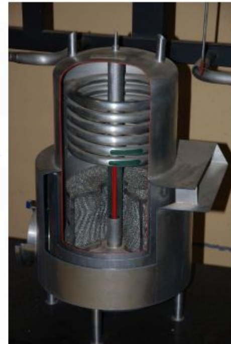
Mockup Cold Trap in Cadarache CEA Sodium School
