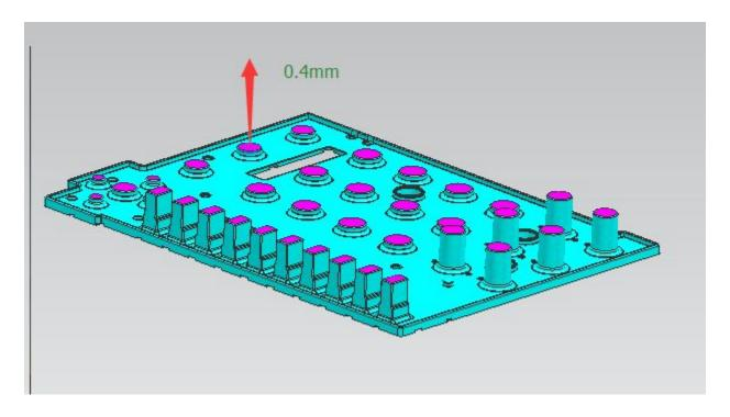
However,we suggust not increase these keys,the plastic keyboards have to decrease 0.4mm if you want to increase 0.4mm for the rubber keypads, therefore, the plastic keyboard will be compaction state during asembling.
