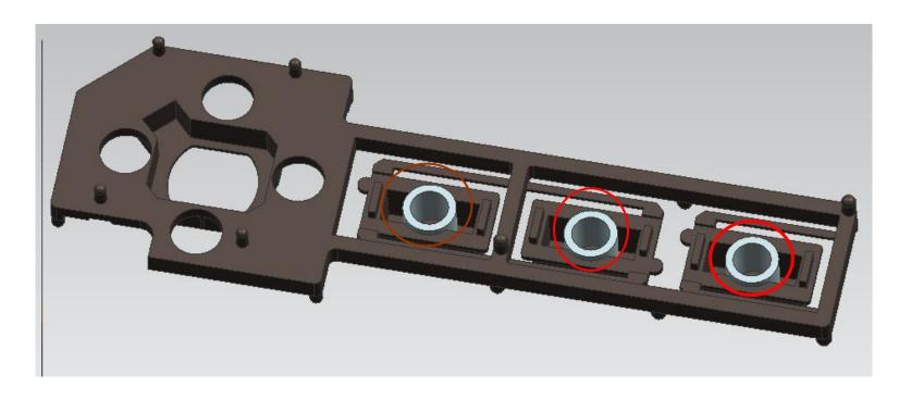
The cross ribs have been changed to round ribs with ¢6.8mm
