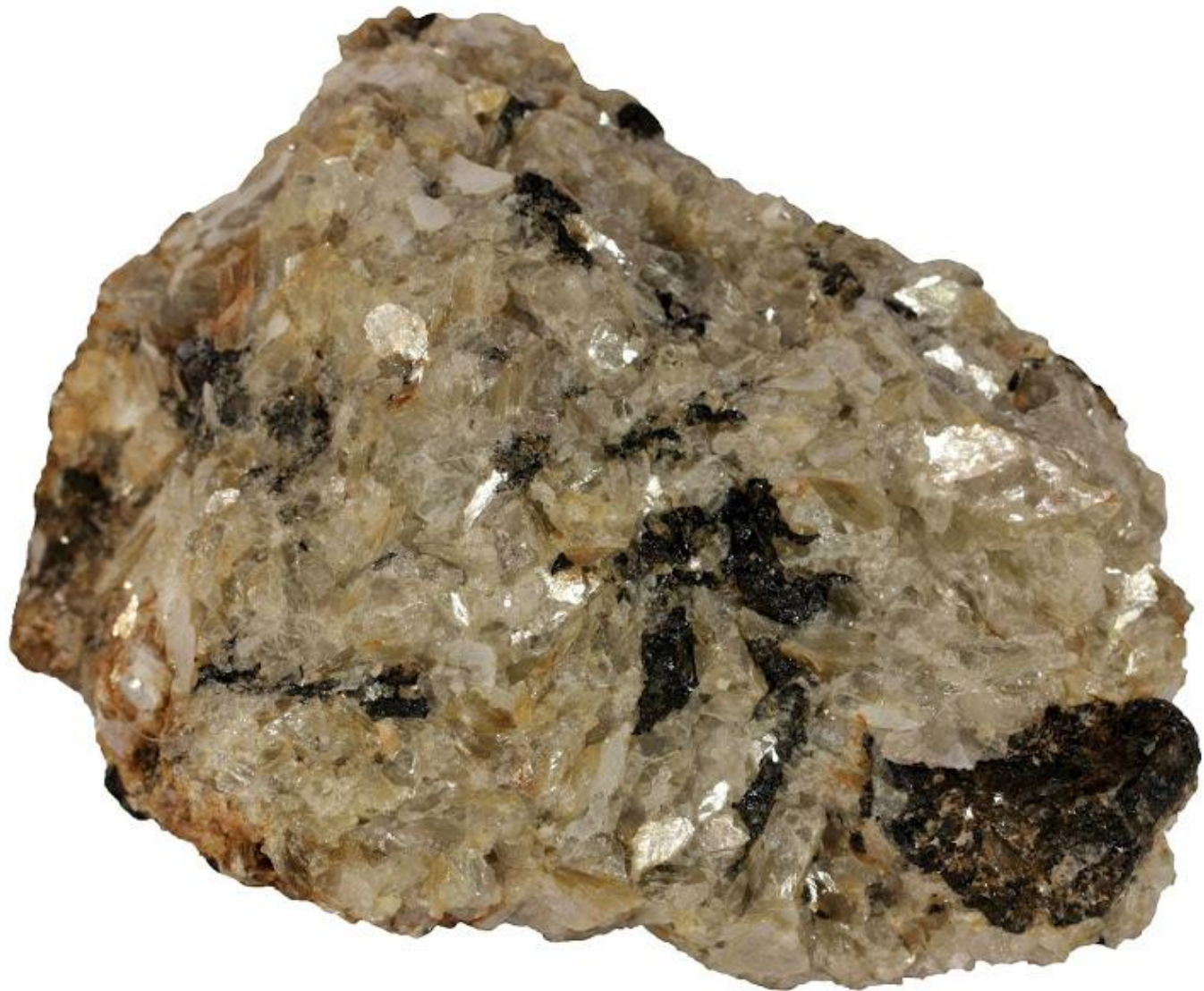
Greisen with cassiterite from Okombahe, Namibia. The width of the sample is 10 cm.
