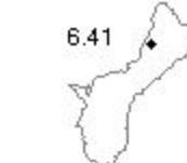
**Average Daily Solar Radiation Per Month****JANUARY**
