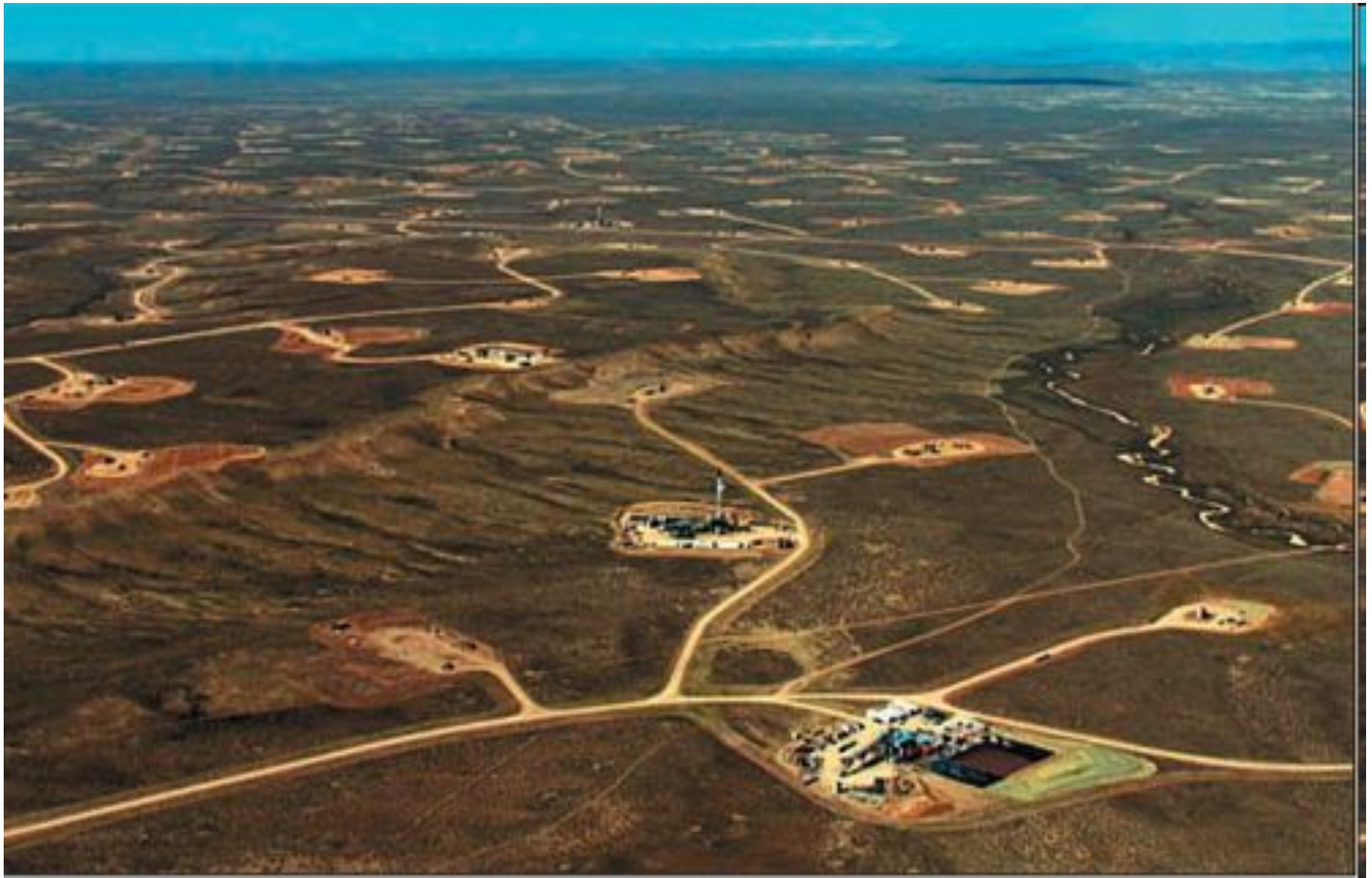
View of 40-acre spacing. Jonah field in Rocky Mountains. Courtesy of www.shaleshock.org
