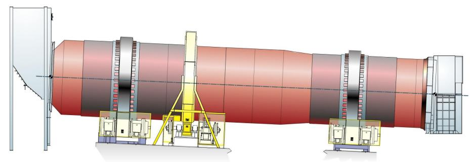
This is basically what a kiln is. The material come in on the left through that shoot and then it moves downwards. The 3 devices around it are different types of "tyres" which basically make it spin, and keeps it up and straight.
