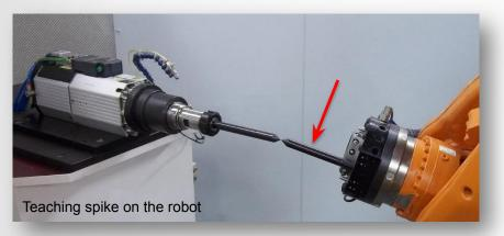
This will give the position of the robot spike tip from the robot flange (6<sup>th</sup> axis) workplane and allow to jog the robot around the robot spike tip.
