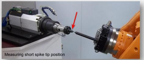
Moving the previously taught robot spike tip against the short probe tip will show, on the robot teach pendant, the position of the short spike tip from the robot world workplane.
