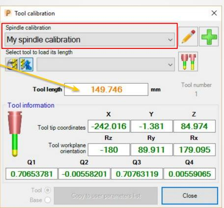
This information should go in the robot controller or in the robot program.
