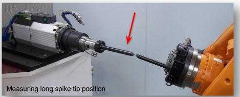
The same as above needs to be done with the long probe... and the coordinate from the world workplane needs to be entered in the spindle calibration form.
