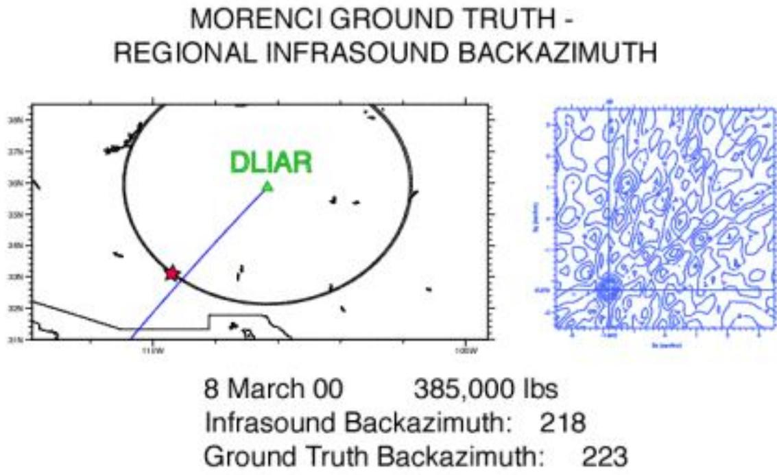
Figure 8: Mining explosions from the hard rock copper mines in southeastern Arizona generate infrasound signals as exemplified by the records from DLIAR in Los Alamos (left). Ground truth for this event was provided by close-in seismic and acoustic records of the blast (left, inset). Frequency wave number estimates were used to make the back azimuth estimate shown to the right.
