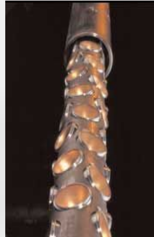
High shot density perforating gun (TCP type)
