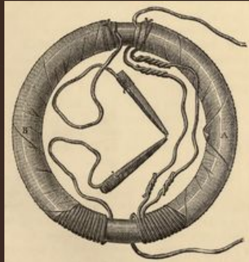
"Faraday transformer": when the current is turned on or off in one winding, the current is recorded in the other.
