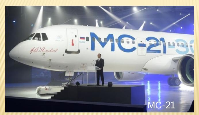
It has a carbon fibre reinforced polymer wing and is powered by Pratt & Whitney PW1000G or Aviadvigatel PD-14 turbofans. With a capacity of 132–163 passengers in two class and up to 6,000–6,400 km range. By July 2018, it had received 175 firm orders and recorded nearly 150 intentions.
