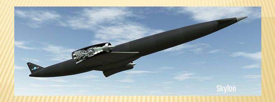
Developed by the British aerospace company Reaction Engines Limited Skylon, 82 meters long and 25 meters wide, it will take off and land on the runway like a "normal" plane, but at the same time it will be able to achieve hypersonic speeds and altitudes of 26 kilometers, switching to oxygen from its own tanks.
