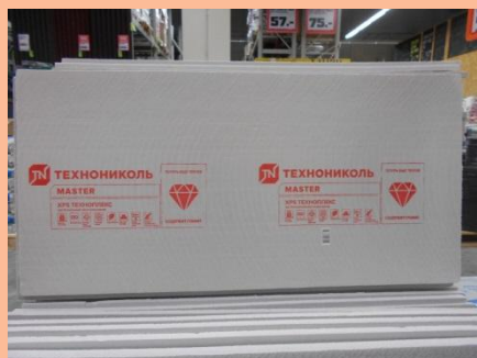
expanded polystyrene "XPS Technoplex 1", 18X0,58X
