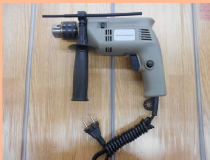
No name PERCUSSION DRILL 500W Voltage: 230V / 50 Hz
