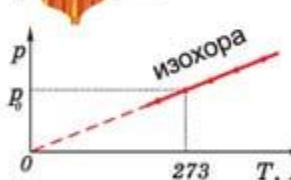
$$\begin{aligned}V &= \text{const} \\ \frac{p}{T} &= \text{const} \\ p &= p_0 \alpha T\end{aligned}$$
