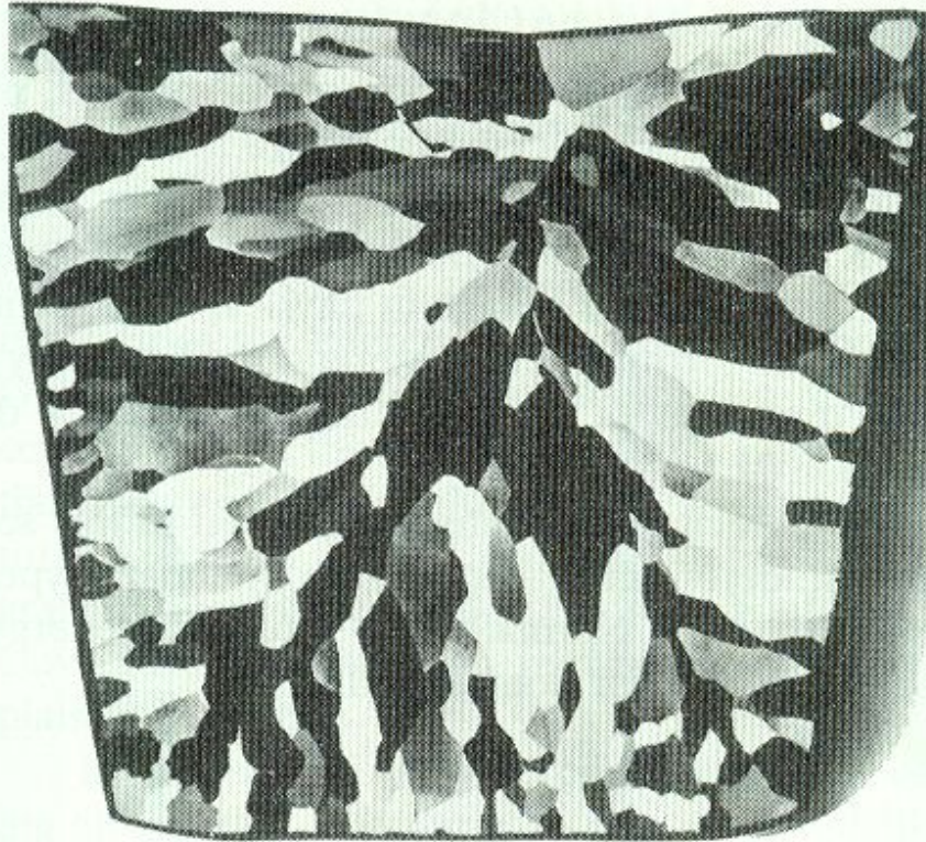
FIGURE 4.10 High-purity polycrystalline lead ingot in which the individual grains may be discerned. 0.7\times . (Reproduced with permission from Metals Handbook , Vol. 9, 9th edition, Metallography and Microstructures , American Society for Metals, Metals Park, OH, 1985.)
