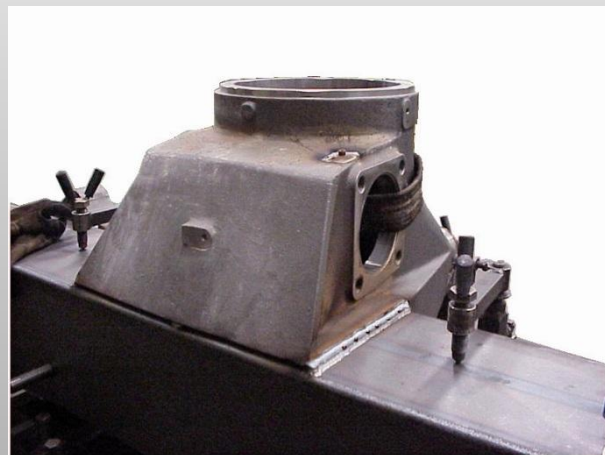
Steel cast support elded welded to the crane crossbar
