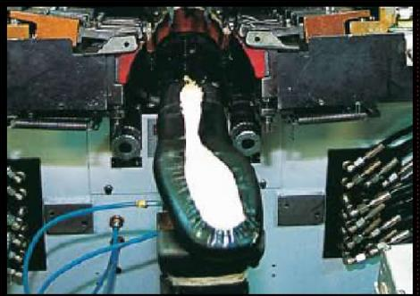
The Machine pulls the upper edges below the insole and glue is applied
