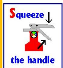
Squeeze the top handle, this depresses a button that releases the pressurised extinguishing agent
