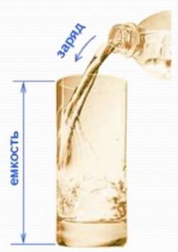
**1 amp** \* **hour** - an electrical charge that passes through the cross-section for one hour in the presence of it in a current of 1 ampere.
