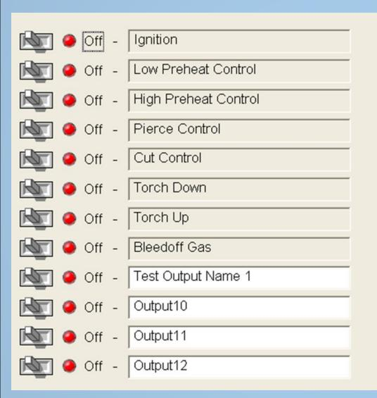
Typical Output layout for OxyFuel Table with Igniters.
