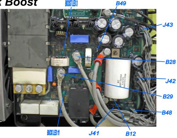
Depending upon the input line voltage, the PFC Control PC Board will very the ON time of the Buck and/or the Boost switches in order to obtain a constant 400 VDC supply.
