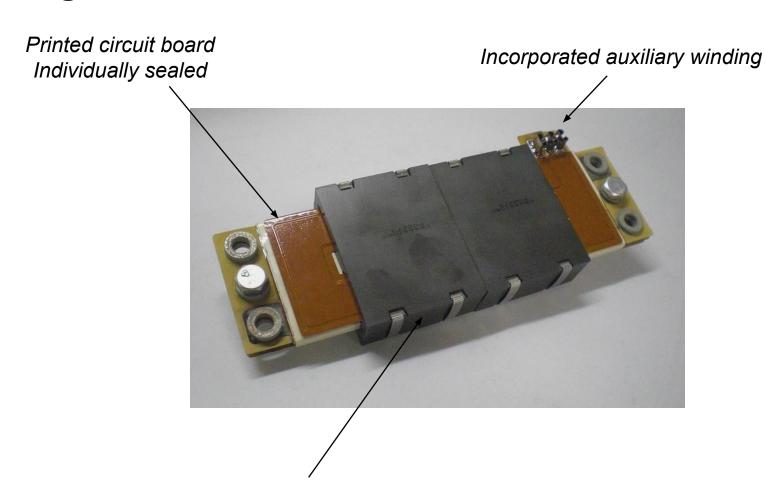
Small footprint allows for mounting directly onto switchboard
