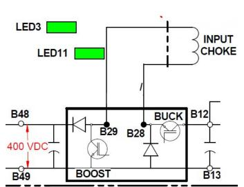
LED3: BOOST IGBT DRIVE LED11: BUCK IGBT DRIVE
