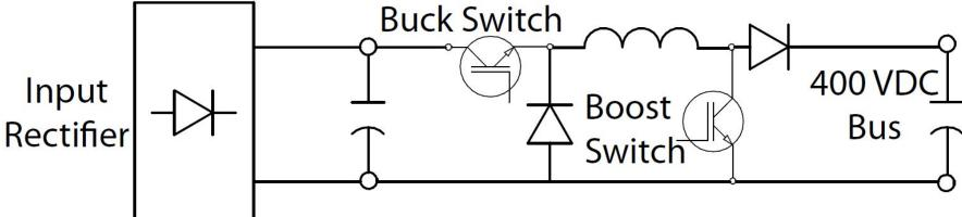
Depending upon the input line voltage, the PFC Control PC Board will very the ON time of the Buck and/or the Boost switches in order to obtain a constant 400 VDC supply.
