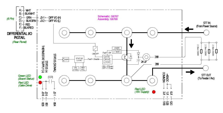
Gate Drive Signal (RS-485 Differential signal from Power Source)
