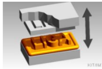
Fig. 36: Moulding for mass replication
