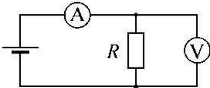
$$R_{\delta} = \frac{U - U_{\delta}}{U_{\delta}} R_{\delta} = (n - 1) R_{\delta}$$
