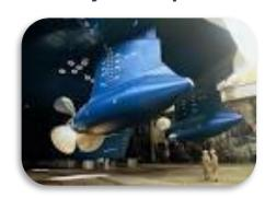
Our calculations show the ability to reduce the motor size from diameter 1800 mm to 1500 -1400 mm.
