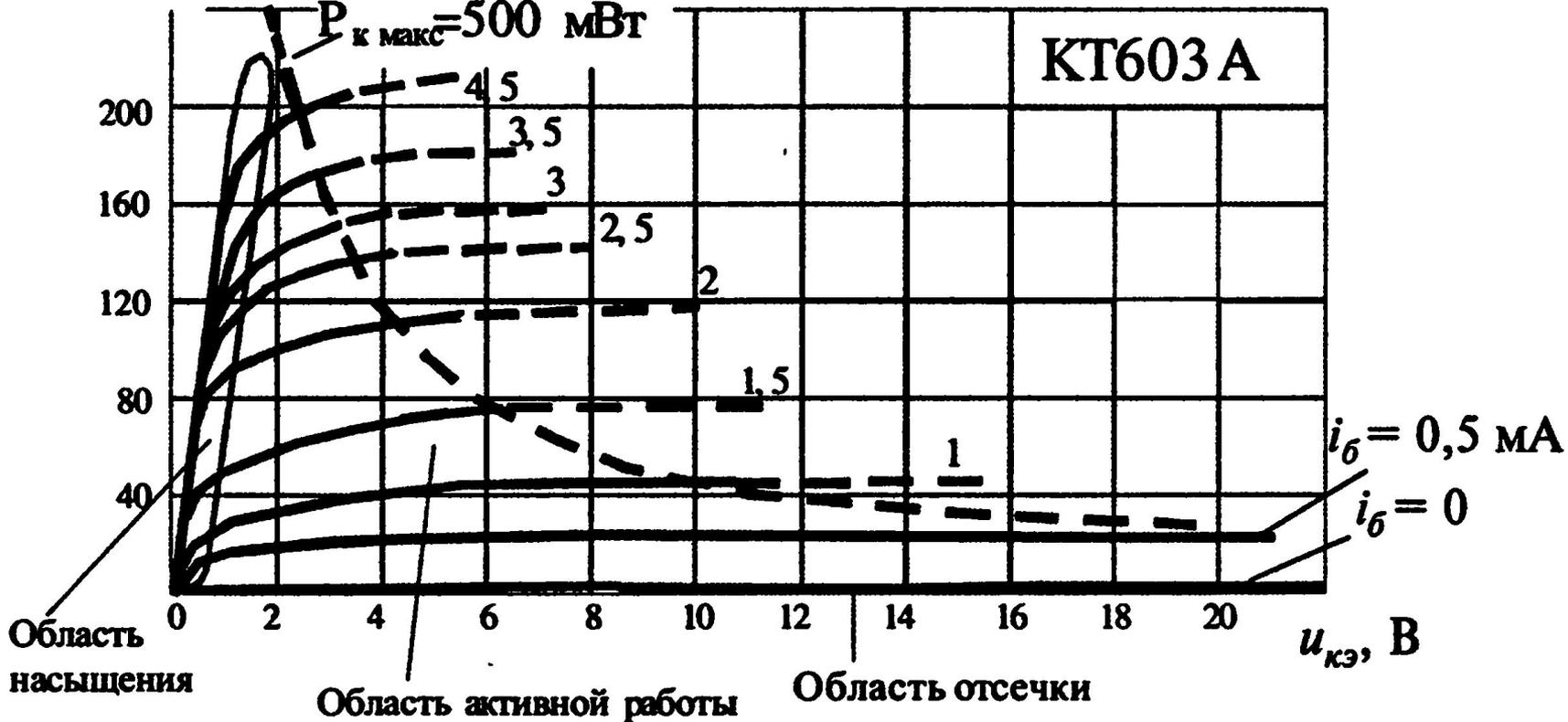
$$h_{21} = \frac{\Delta I_{\text{вых}}}{\Delta I_{\text{вх}}} = \frac{\Delta I_K}{\Delta I_B}$$
