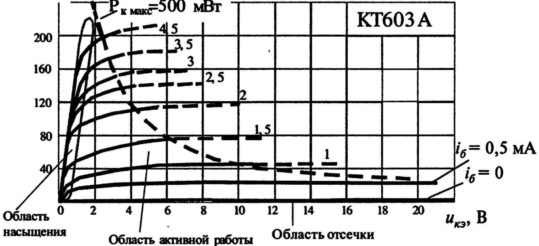
$$h_{22} = \frac{\Delta I_{\text{вых}}}{\Delta U_{\text{вых}}} = \frac{\Delta I_K}{\Delta U_{KЭ}}$$
