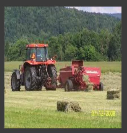
Most modern pick-up balers are driven by an engine mounted on the baler, or by the engine of the towing tractor. This method is known as power take-off. It is power achieved by means of a universal jointed coupling from the power take-off shaft of the tractor to the baler.
