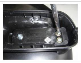
4<sup>th</sup>: dismantle pressure release valve base and core.
