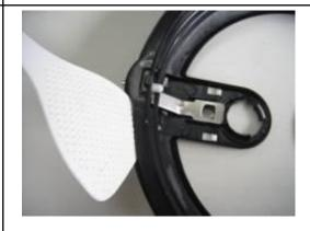
8<sup>th</sup> step: separate cover lining and cover and dismantle pushrod assembly
