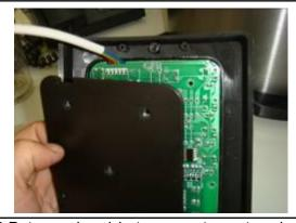
10.Put your hand between outer pot and outer shell to pull to separate outer shell from outer shell cover button.
