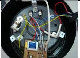
8.Remove control box from outer shell and 5 screws on control box cover, then control board assembly can be exchanged.
