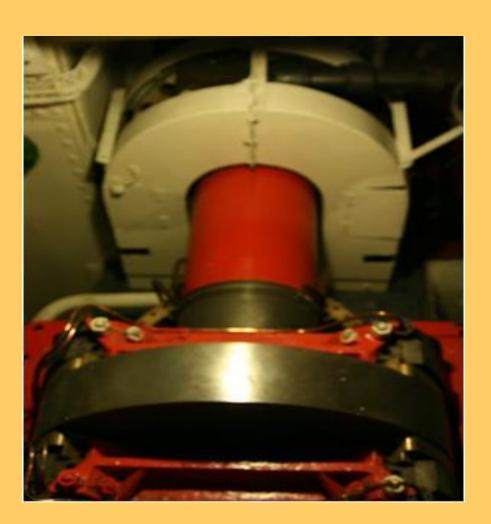
The thrust block takes up the propulsion forces of the screw and conveys them to the hull of the ship.
