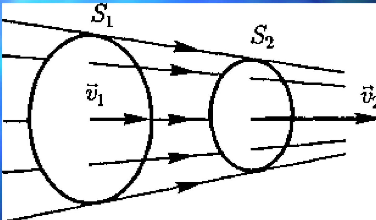
$$S_1 v_1 = S_2 v_2 = \text{const.}$$
