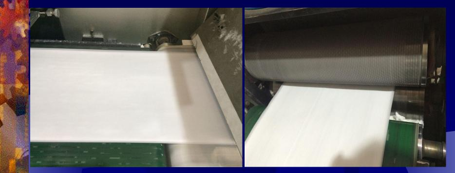
two layers of tissue with the fluff pulp fiber in between, is being embossed—forming the core
