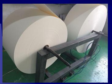
the fluff pulp rolls are loaded on the machine and broken up into powder fibers by the hammer mill
