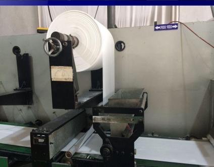
the back-sheet and top-sheet tissues carry the fluff pulp fiber and transfer it to the next step, embossment
