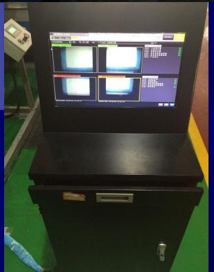
the Spots monitor screens the entire long sheet on line. The alarm goes off if any foreign material is detected.
