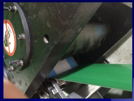
The sheet is transferred to the second cutter, being cut to the designed size and folded at the same time.
