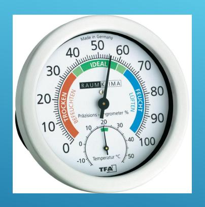
Another tool we can use is a hygrometer. This tells us how much moisture is in the air.
