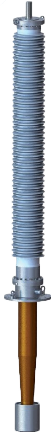
Air — Oil bushing for power transformers Voltage: 252 kV Current: 1250–2000 A Insulation: RIP
