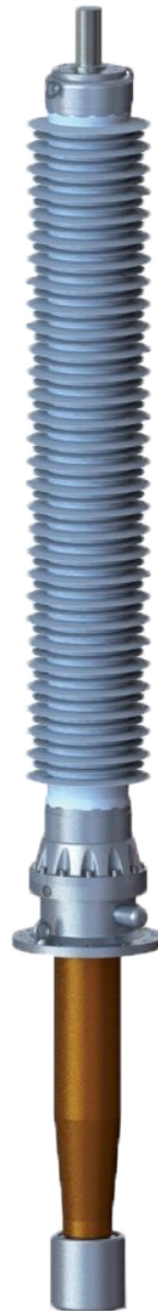
Air — Oil bushing for power transformers Voltage: 145 kV Current: 1250 A Insulation: RIP
