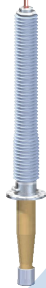
Air-Oil bushings for power transformers and shunt reactors Voltage: 12-1200 kV Current: 315-5000 A Insulation: RIP or RIN (up to 550 kV)
