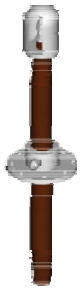
Oil-Oil bushings for cable connection of transformers Voltage: 72.5-550 kV Current: 630-1000 A Insulation: RIP or RIN
