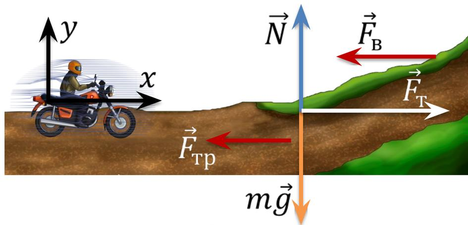
$$F_{\text{Т}} = F_{\text{Тр}} + N + mg + c v^2$$
