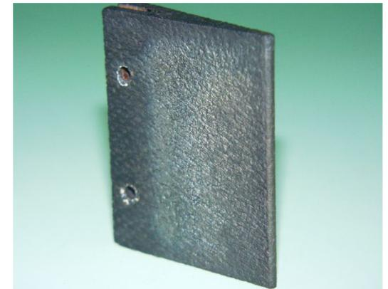
Fig 9 – Leading edge samples (0.75 mm radius ) after test
