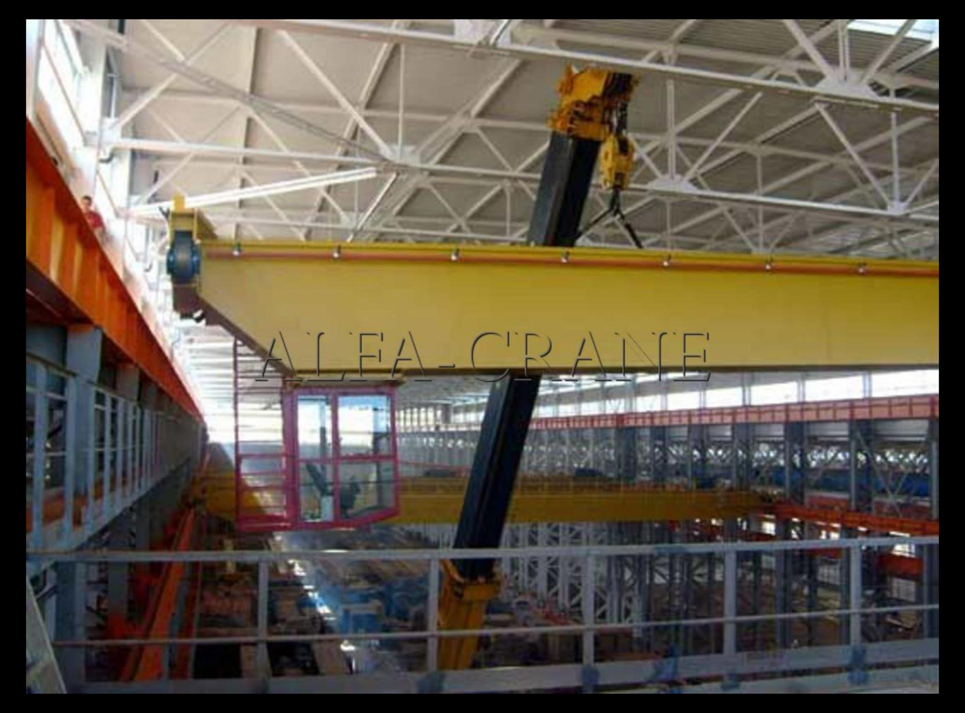
A large yellow overhead crane is mounted on a white steel truss ceiling in a warehouse. The crane has a red control cabin and a black vertical support column. The warehouse floor is filled with various items, and there are metal railings in the foreground. The text "ALFA-CRANE" is overlaid on the image.
