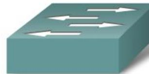
The frame is forwarded through the switch before the entire frame is received.
