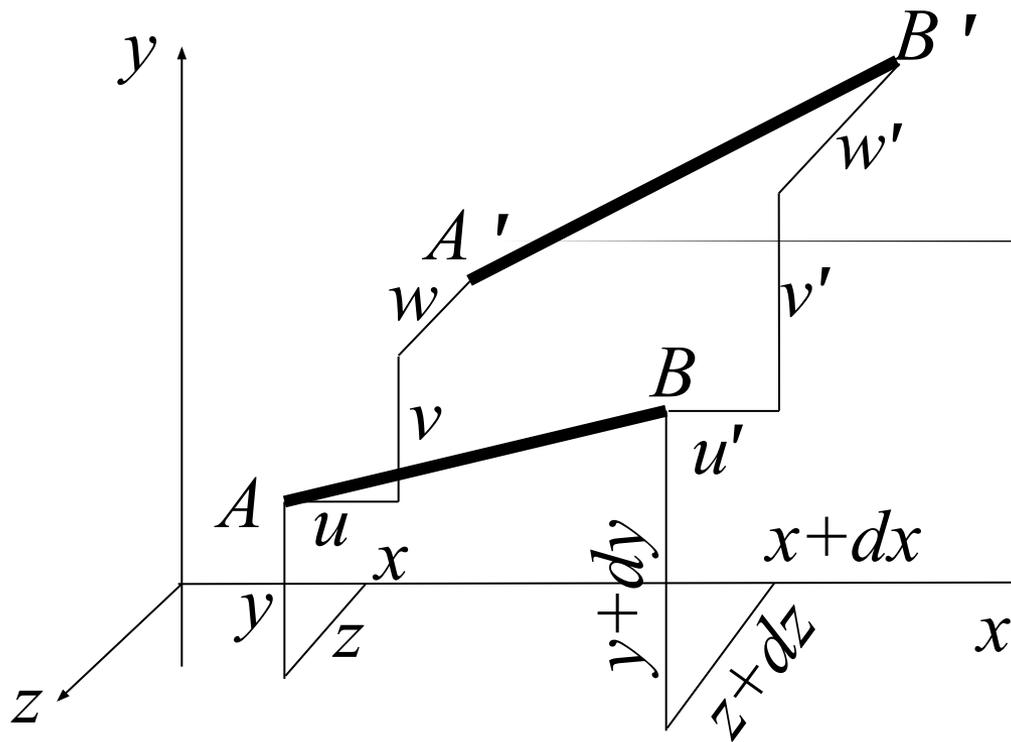
$$\left[ \begin{array}{l} u' = u + \frac{\partial u}{\partial x} dx \\ v' = v + \frac{\partial v}{\partial x} dx \\ w' = w + \frac{\partial w}{\partial x} dx \end{array} \right.$$
