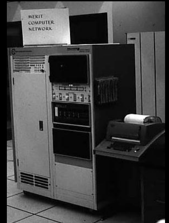
Merit PDP-11 Merit PDP-11 based Primary Communications Processor (PCP) at the University of Michigan, c. 1975
