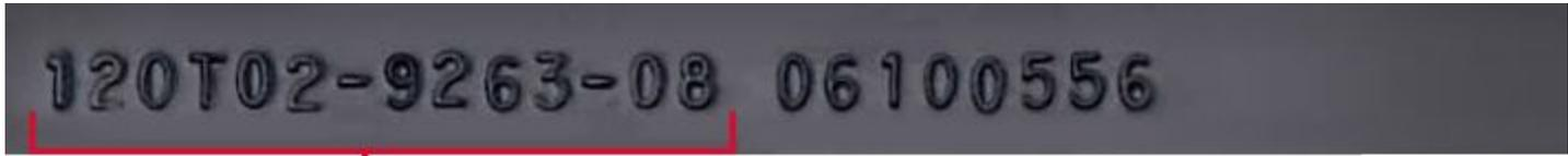
A photograph of a dark metal surface with a stamped engine model number. The number is '120T02-9263-08 06100556'. A red bracket is drawn under the first part of the number, '120T02-9263-08', to indicate it is the model number.
