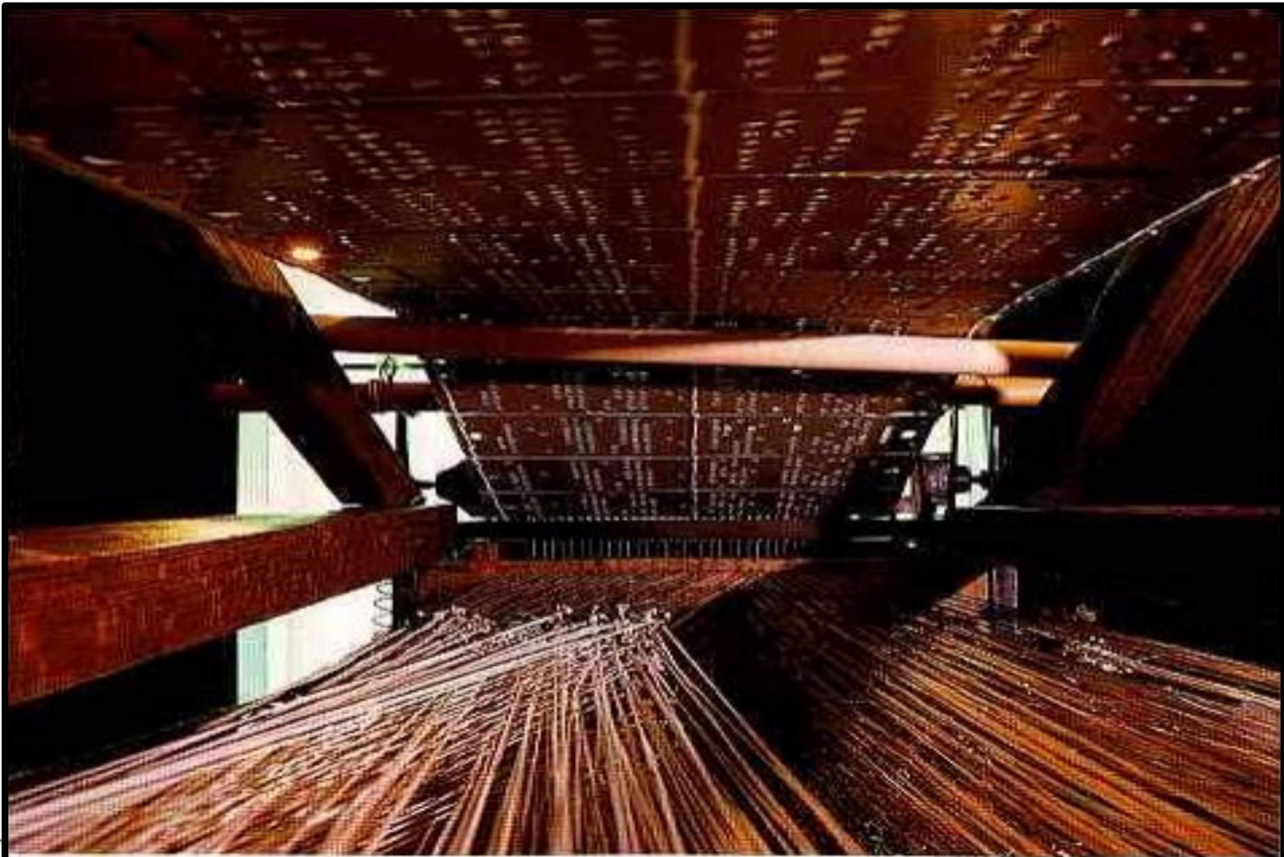
Jacquard's Loom showing the threads and the punched cards
