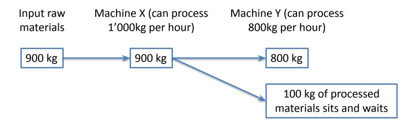
Shall we keep Machine X working on its maximum?
