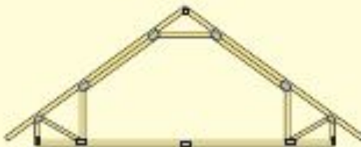
Attic frame truss
