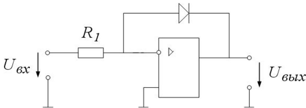
$$U_{\text{вых}} = \frac{1}{a} \cdot \ln \left( \frac{U_{\text{вх}}}{I_0 \cdot R_1} \right)$$
