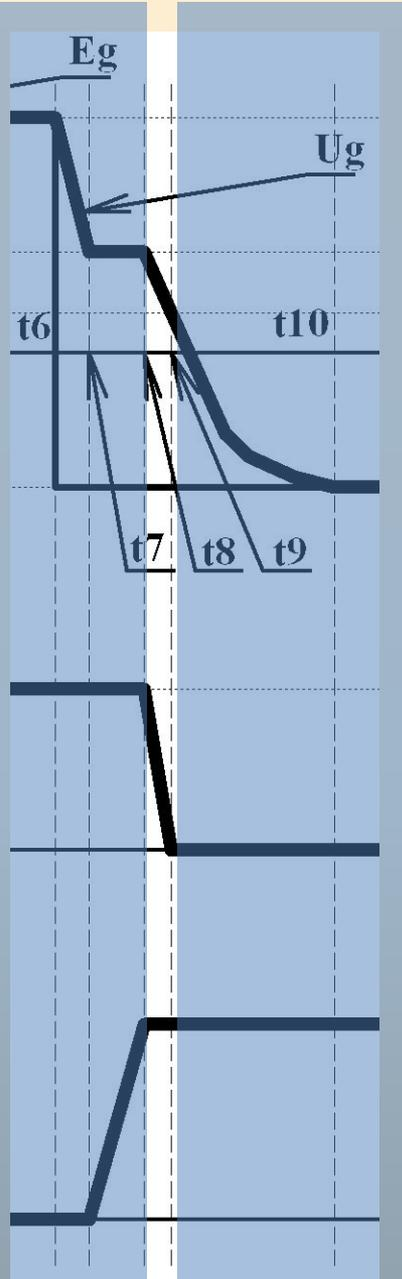
$$I(t) = J - [J + S \cdot (V_{g0} - U_{g-})] \cdot \frac{t - t_8}{R_g \cdot (C_{gs} + C_{dg})}$$
