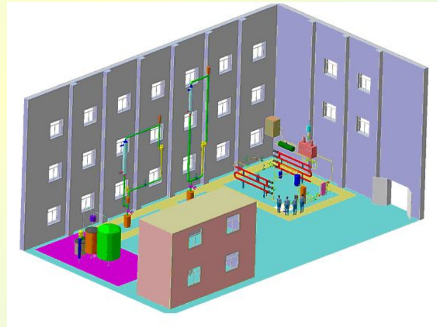
the illustration of Lead-bismuth experimental loops for KYLIN-I and KYLIN-II
