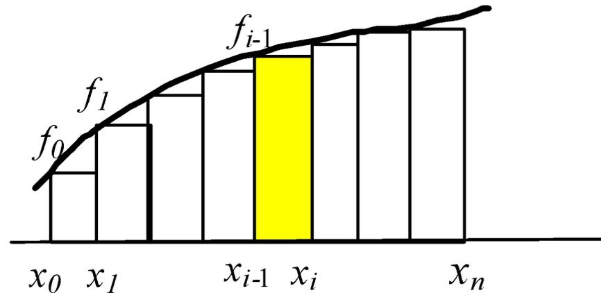
$$I_{l\_pr} = f_0(x_1 - x_0) + f_1(x_2 - x_1) + \dots + f_{n-1}(x_n - x_{n-1}) = \sum_{i=1}^n f_{i-1}(x_i - x_{i-1})$$
