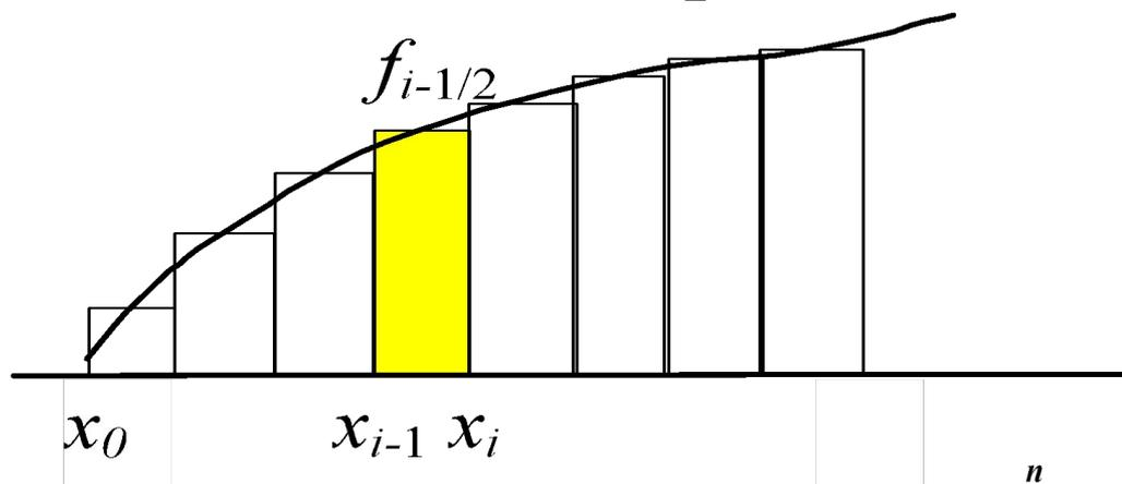
$$I_{c\_pr} = f_{1/2}(x_1 - x_0) + f_{3/2}(x_2 - x_1) + \dots + f_{n-1/2}(x_n - x_{n-1}) = \sum_{i=1}^n f_{i-1/2}(x_i - x_{i-1})$$
