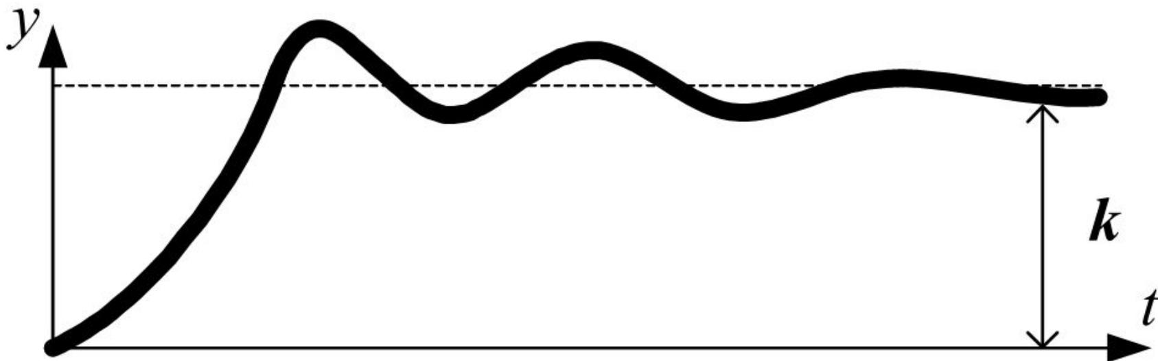
$$W_{\text{кол}}(p) = \frac{K}{T_2^2 p^2 + T_1 p + 1}$$
