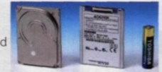
Toshiba's 1.8" hard drive; mini hard drives are used in small gadgets, such as PDAs and wristwatches
