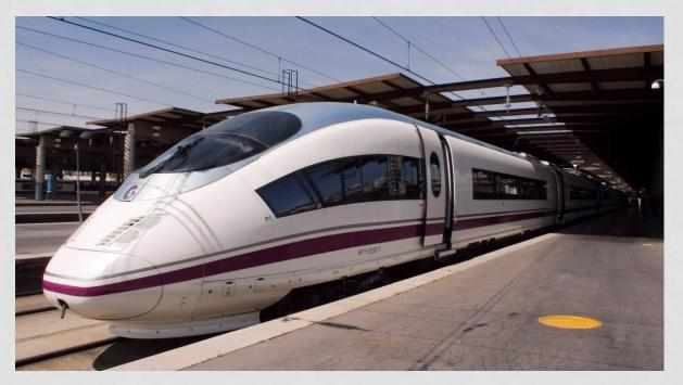
Velaro E, designated as AVE S 103 in Spain, is the fastest series-production high-speed train in the world. It achieved a whopping speed of about 400kmph during its test trips in Spain.
