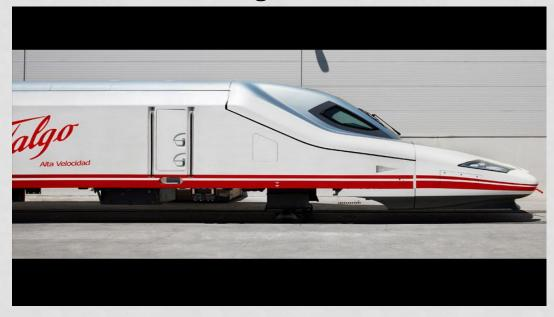
Talgo 350, which initially entered service with the name RENFE AVE Class 10, achieved a maximum speed of 365kmph during its trial run. The train has a maximum operational speed of 350kmph.
