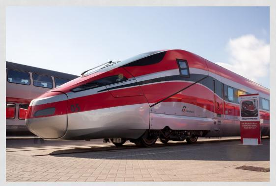
Elettro Treno Rapido 500 (ETR 500) Frecciarossa trains entered into service in 2008. The trains are designed for a maximum speed of 360kmph and currently run at 300kmph on high speed lines.
