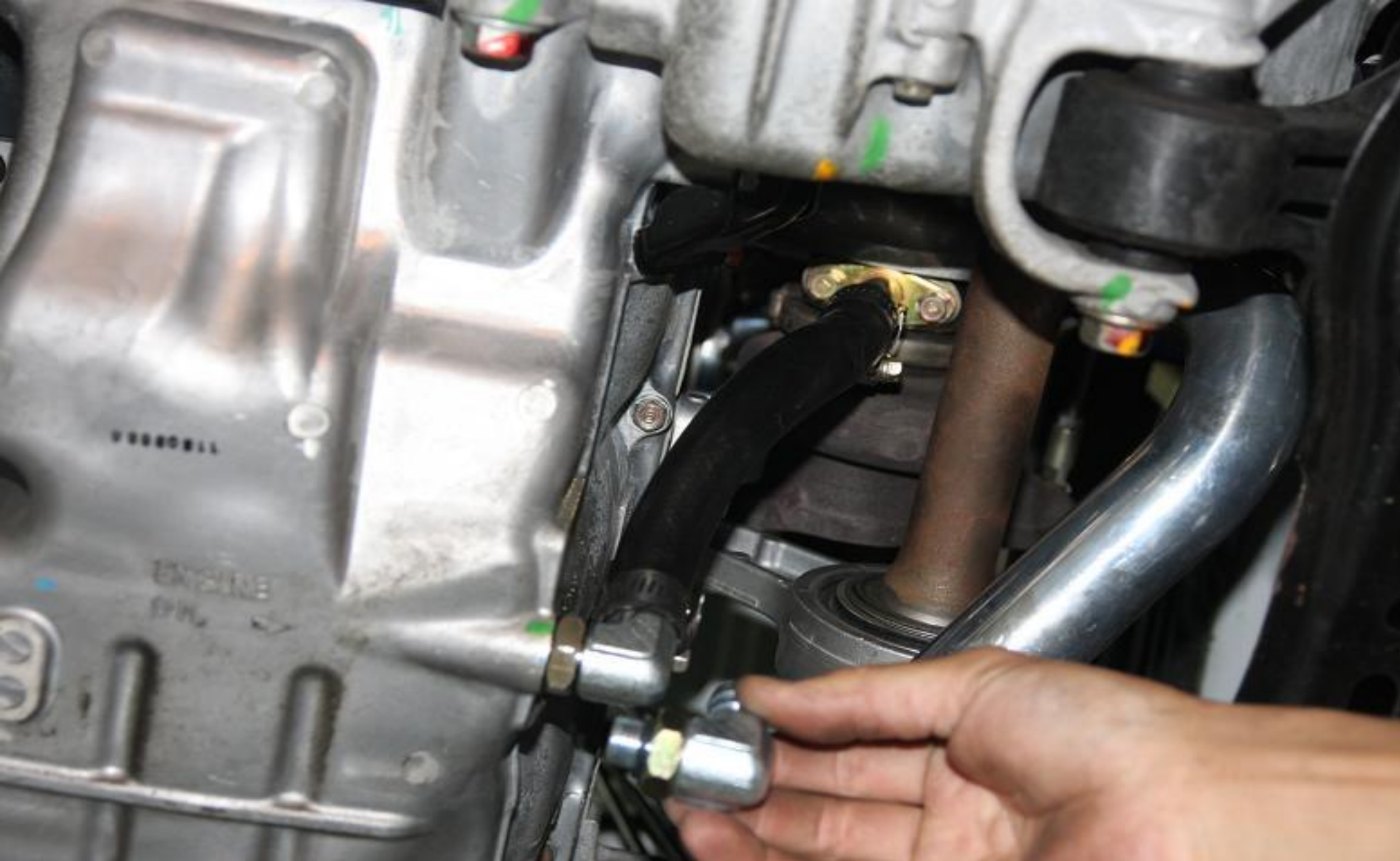
Install oil drain pipe
