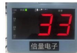
4. The external display for domestic market Single line, only display sheet or total value
