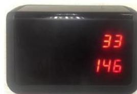
3. RGD external display 2 lines display, the 1 st line displays sheet, the 2 nd line displays total value.
